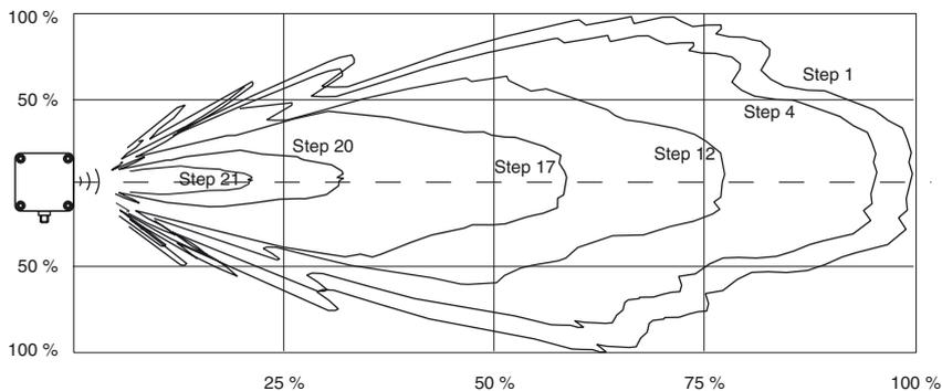
**Sensitivity adjustment for suppression of disturbing targets**
